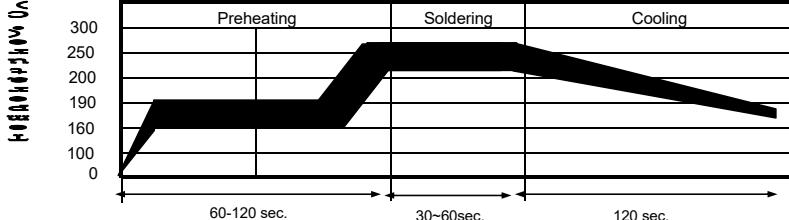
Recommended reflow methods: IR, vapor phase oven, hot air oven.
